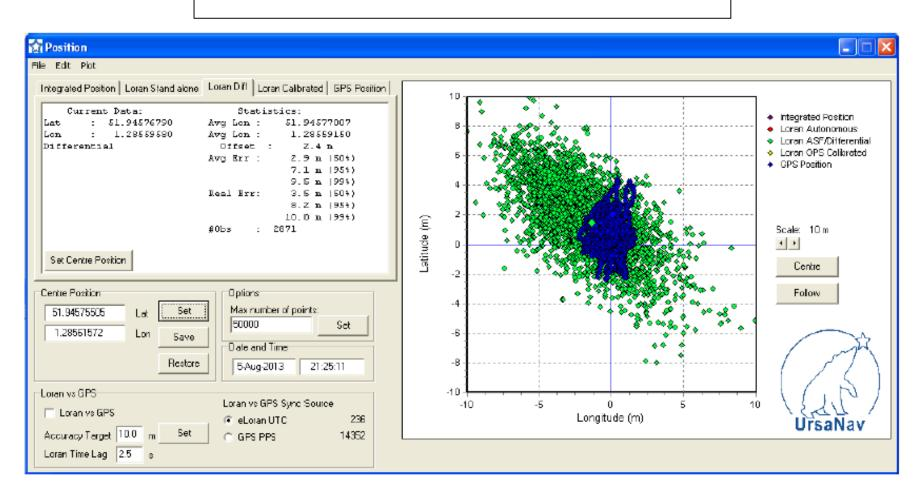
Differential eLoran. Offset 2.4 m (< 8 feet). Error 7.1 m (95%) from surveyed position. Note: 2.4 m equates to less than eight nanoseconds.
