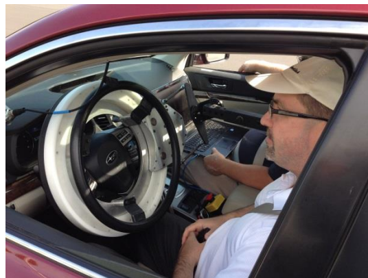
Figure 4: The Test Vehicle Drop-In Actuator Kit can convert any vehicle into an automated system within 30 minutes
