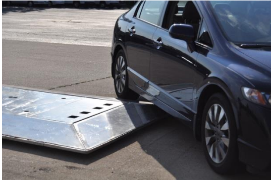
Figure 5: The Target Robot is designed to sustain a run-over by SUVs and tractor trailers
