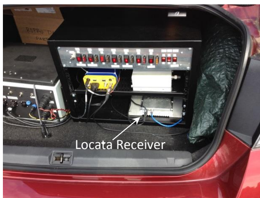
Figure 6: A Locata Receiver, installed as an integral part of the DAK, provides position accuracy to <10cm
