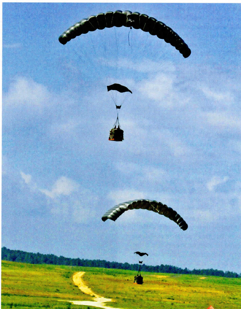
A GPS-GUIDED Joint Precision Air Drop System (JPADS) 2K parachute flies to its ground target. The U.S. Army is testing visually-aided navigation systems for JPADS use in GPS-denied environments such as canyons and cities.
