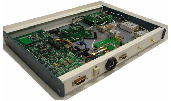
Fig. 9. The Cornell GRID receiver – the hardware platform for the receiver-spoofers.
