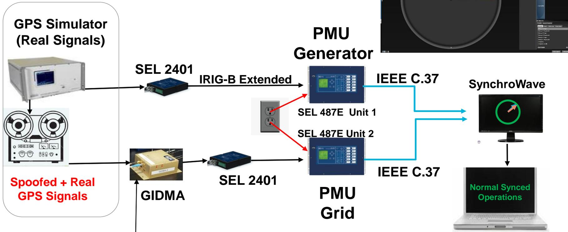
**Detects GPS Spoofing and blocks fake signal from entering the receiver**
