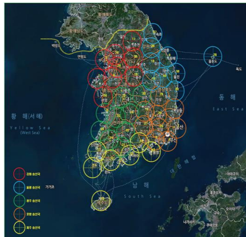
Number of “differential eLoran stations” proposed by South Korea attempting to provide “20 m accuracy” (Page 9, Appendix A)
