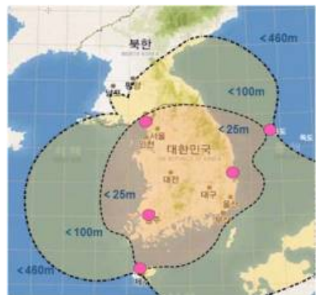
Projected accuracy and coverage of Korea's eLoran network. Ministry of Oceans and Fisheries of Korea (Click image to enlarge.)
