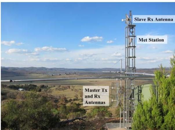
Figure 2. NTF South site—overlooking the rest of the NTF.
