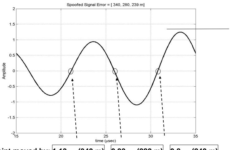
Tracking point moved by: 1.13 μs (340 m) 0.93 μs (280 m) 0.8 μs (240 m)
