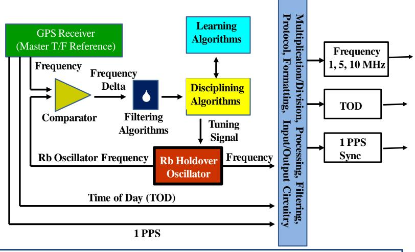
It is the TFS, not the GPS Receiver alone, that should be considered as the building block for timing, frequency, and time-of-day services.
