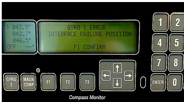
Figure 8 : Photograph of the gyro-compass in an alarm mode following the loss of GPS.
