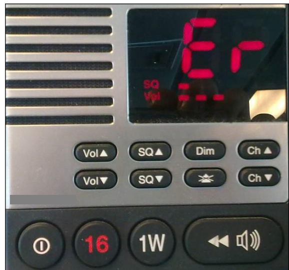
Figure 4: The vessel's VHF transceiver provides an audible and visual alarm when GPS is not available.
