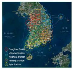
Figure 6: Selected locations for the 43 differential eLoran stations [1]. The radius of each circle is 30 km.
