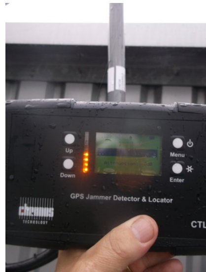
Figure 2: CTL3520 identifying the rogue antenna at LD4
