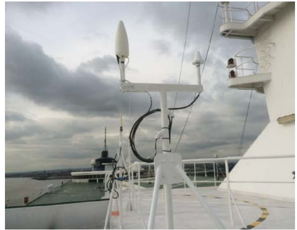
Figure 14. Antenna Installation on the Pride of Hull (eLoran on the left, GPS on the right)
