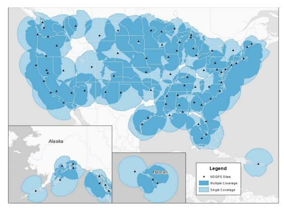
Figure A-6 NDGPS Signal Coverage
