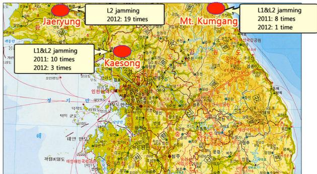
Figure 1: North Korean GPS jamming and jammer locations in 2011 and 2012 [1]
