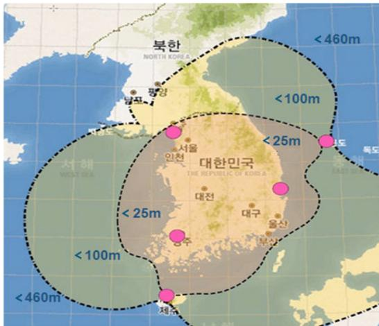
Figure 4: Simulation result of the expected accuracy and coverage of the Korean eLoran system provided by ANSE Technologies [1]
